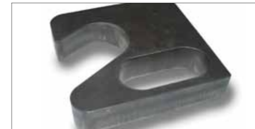
Example for 20mm cutting with Air/Air on Mild Steel
